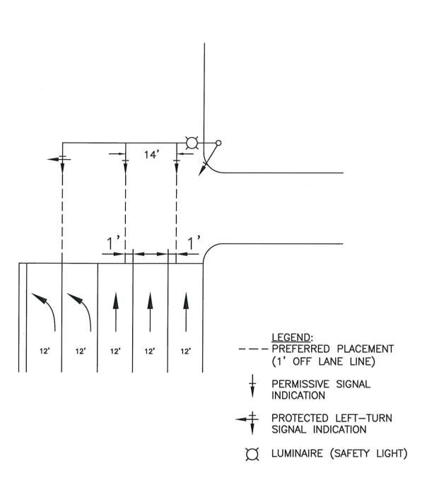
NOTE: TRAFFIC ENGINEER SHALL DESIGN TRAFFIC SIGNAL LOCATION AND ORIENTATION BASED ON THE OPERATION AND SAFETY OF EACH INTERSECTION. THE DESIGN SHALL BE APPROVED BY THE CITY ENGINEER.
