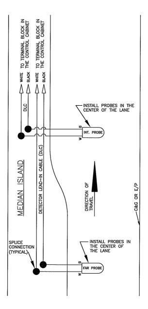
SINGLE LANE MAGNETIC PROBE INSTALLATION
